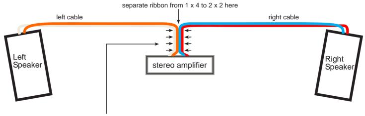
keep the ribbon together from amplifier level to floor level to retain cable directionality
