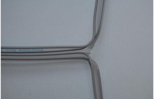
SEPARATE THE RIBBON BY TEARING JUST ENOUGH TO CONNECT THE LEFT AND RIGHT SPEAKERS
