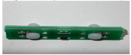
Undo the two nylon screws/nuts to separate the cable clamp pcb as shown.
