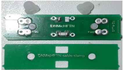
Note the position of the HFTN relative to the plugs. The end marked "to plug" must face the end of the cable where the plugs are fitted.
