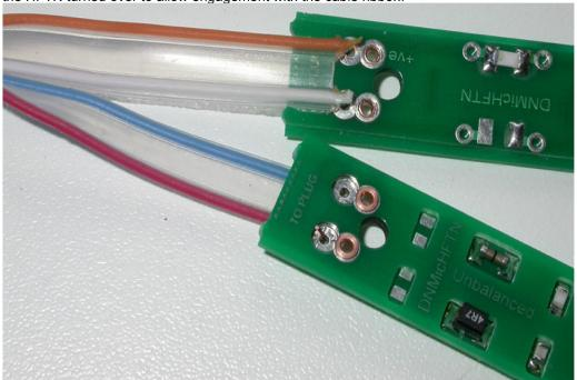
Solder each conductor to its corresponding end pad on the HFTN main pcb. The diameter of the conductor will lie on the surface of the pcb but the bulk of the insulation material will lie between the two extended forks of the main pcb.
