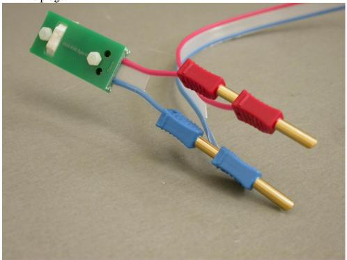
The illustration below shows where the HFTN is connected to the speaker cables.
