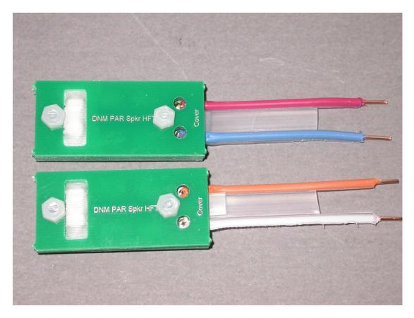
The DNM RF termination system, named "High Frequency Termination Network" (**HFTN**), is a precision circuit that controls the radio frequency (RF) load presented by the cable to the amplifier. The HFTN terminates the cable at the radio frequencies that are generated by the amplifier's feedback system.
