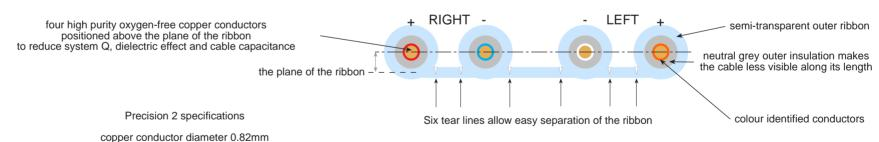
resistance 0.03 Ohms/metre capacitance 17pF/metre inductance 1.03uH/metre
